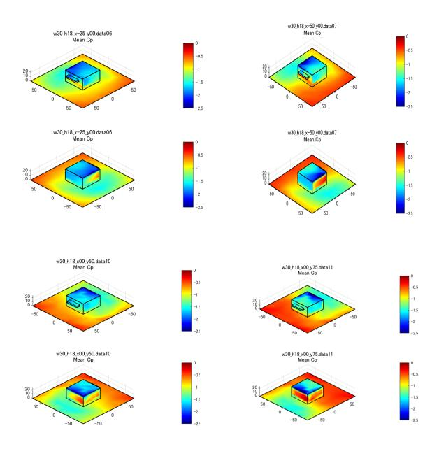
Figure-2 Mean Cp distribution on the building model, canopy and surrounding for 29.8 mm canopy fixed at ¾ height from the surface, when tornado moves in x and y direction
